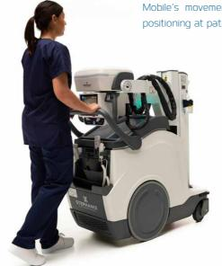
**Movix DReamy** rear diameter load wheels, as well as front steering wheels featuring shock absorbing springs help tp cross obstacles such as elevator threshold.
